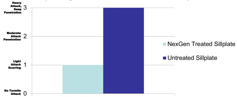
Formosan subterranean termite attack is strongly resisted on NexGen treated sill plates while untreated sill plates show no resistance.
