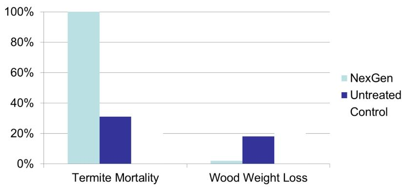
Mortality and weight loss tests demonstrate NexGen's resistance to Formosan subterranean termites. 100% mortality = 0% survival.
