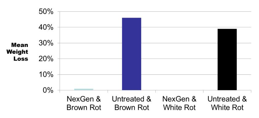
Weight loss due to fungal degradation of wood-based composites is an important concern for the structural integrity of the material used in the field.
