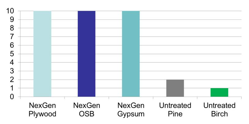
Inoculated with fungi and exposed over a 5 week incubation period, NexGen treated samples show no fungus growth (10 = No Mould Growth, 1 = Total Mould Growth).
